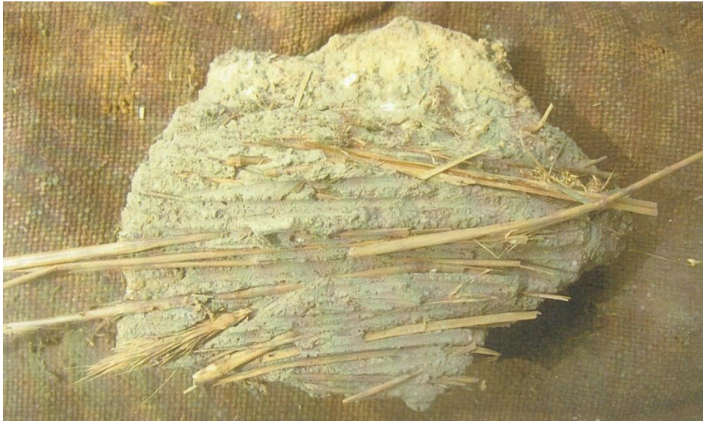
A piece of “brandsolder” material found in the ceiling. The wheat oar still in-tact. The construction of this building dates to c1780. The archaeologist found a whole hessian bag (shown behind the material), in the loft. It appeared to have contained a powdery substance.
